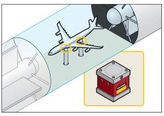
Ideal solution to measure lift, drag, and side force in wind tunnel applications.
