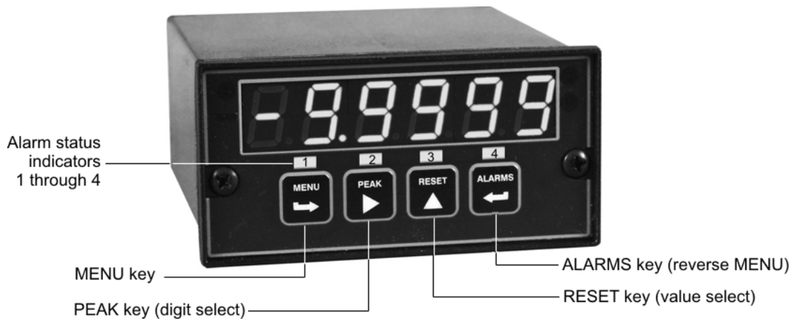
Meter Front Panel
