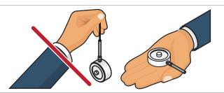
2. Monitor sensor output for effects on zero output during installation to avoid damage.
