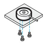
**3.** Retain with set screw, hand tighten to prevent overloading the sensor
