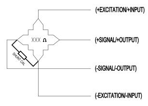
FOR POSITIVE OUTPUT DURING SHUNT CALIBRATION, RESISTOR MUST BE CONNECTED ACROSS -EXCITATION AND -SIGNAL
