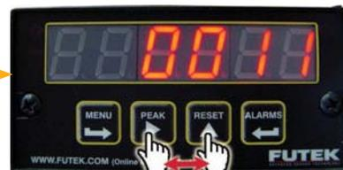
5. Hit **PEAK** button once to show value. Then, hit **PEAK** button again to switch between the digits and **RESET** button to change the number until the value is set to **0011**.
