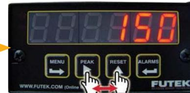
2. Hit **PEAK** button once to show value. Then, hit **PEAK** button again to switch between the digits and **RESET** button to change the number until the value is set to **150**.
