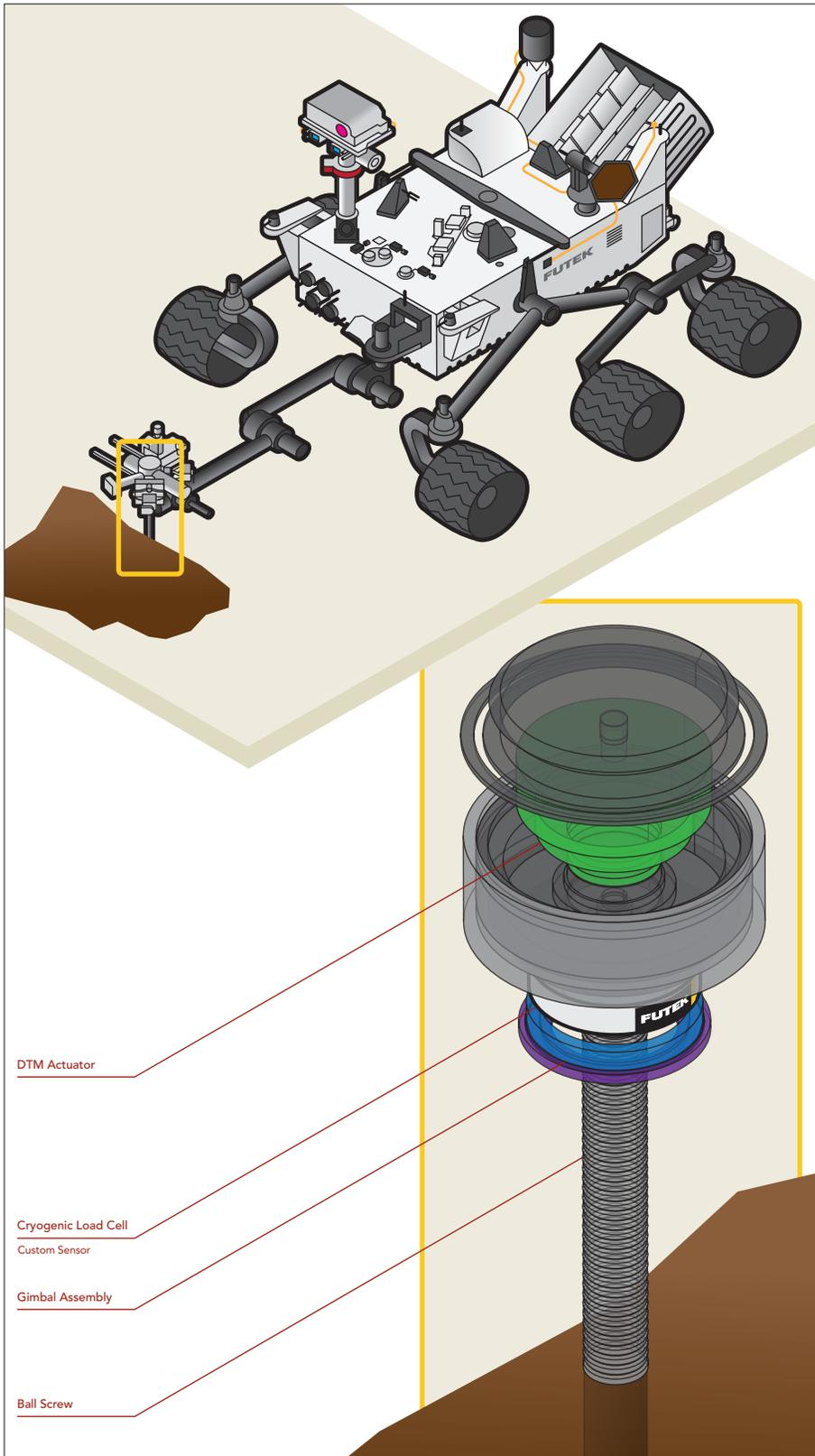
The NASA/JPL rover Curiosity, landed on Mars in August 2012 with the mission to explore Martian terrain. FUTEK developed two unique sensors for the project that operate around the clock, within temperature cycles from 23°F to as low as -124°F.
