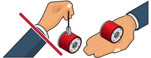
2. Monitor sensor output for effects on zero output during installation to avoid damage.
