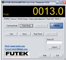
**TEDS (IEEE1451.4) Indicator-** (Available when TEDS option card is installed) When the TEDS icon is dark blue this means there is not a TEDS compliant sensor connected to the display and may require manual entry of the data to set up the display and sensor.
