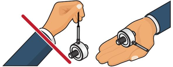
2. Avoid over torque during installation.
