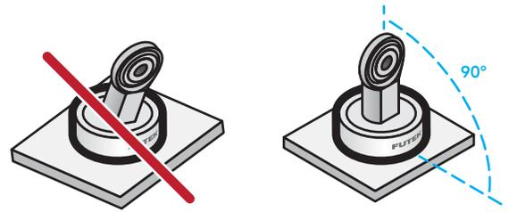
2. Loading must be flat and in-line when compensating linkages are not used
