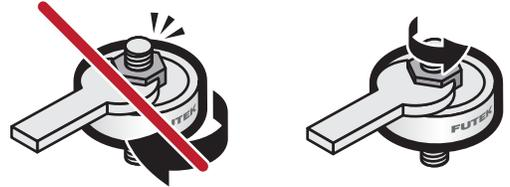
3. Monitor sensor output for effects on zero output during installation to avoid damage.
