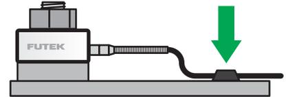
4. Avoid bending the strain relief. Bends in the cable should not exceed a radius of 10 times the diameter of the sensor cable for dynamic, or moving, applications. When permanently routing a cable in a static installation, the minimal bend radius should not fall below 2-3 times the diameter of the cable.
