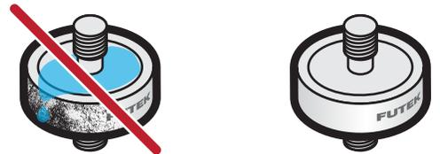
5. Avoid utilizing sensor cover to twist sensor into place.
