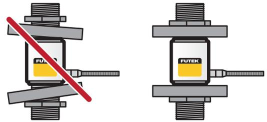
4. A locknut, or jam nut, can be used to help limit the torque into the sensor as well as improve the load distribution in the thread joint which in turn improves the sensor's repeatability.
