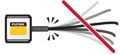
2. Properly secure sensor cable to limit cable movement influence
