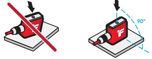
2. Loading must be flat and in-line when compensating linkages are not used
