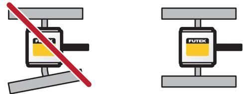
4. Locknut/jamnut can be used to help limit torque. Additionally, this improves repeatability by distributing the load in the thread joint.
