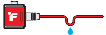
4. Avoid bending the strain relief. For dynamic (moving) applications, bends in the cable should not exceed a radius of 10 times the diameter of the sensor cable. Bends should never exceed a one-time, static, permanent bend of two to three times the diameter of the cable.
