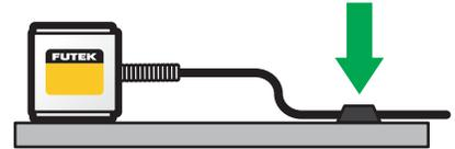
3. In an environment with a high amount of moisture or humidity, create a drip loop on the cable to prevent any water from flowing into the sensor.
