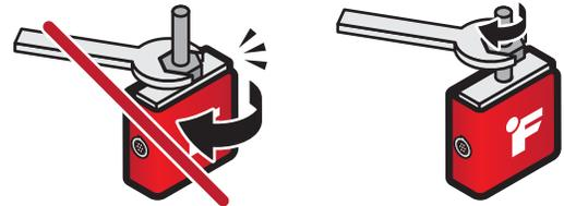
3. Thread the fixture into the sensor. Threading the sensor into the fixture can apply torque that may damage sensor
