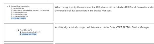
If Windows incorrectly sees the USB device under Device Manager it may be necessary to uninstall the other device, disconnect the FUTEK USB instrument, and re-install the FUTEK FTDI USB driver, and re-plug in the USB device.
